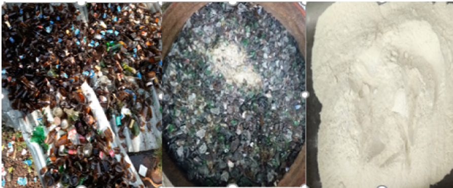
(a) Waste Glass before crushing (b) Small sized Glass Culets (c) WGP after crushing
