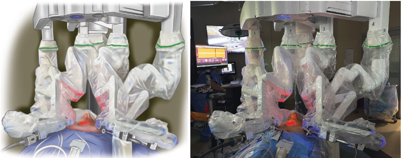
Fig. 13.2 Robot arms are widely spaced, providing an ideal triangulation, depth perception, and working space. Robot arm collision is minimized
