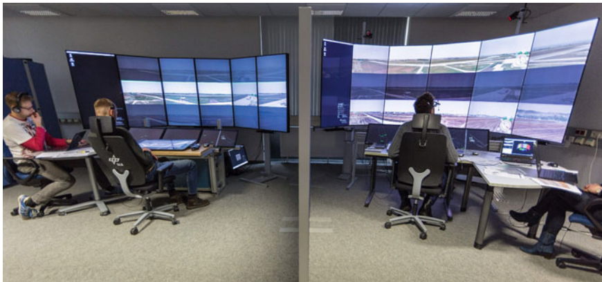
Fig. 1 Multiple remote tower module (MRTM) as used in the study (two active ATCOs with an observer right beside them)
