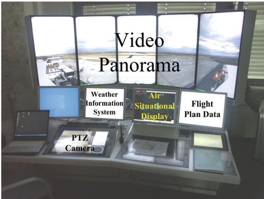
Fig. 2 CWP-remote at the airport Erfurt
