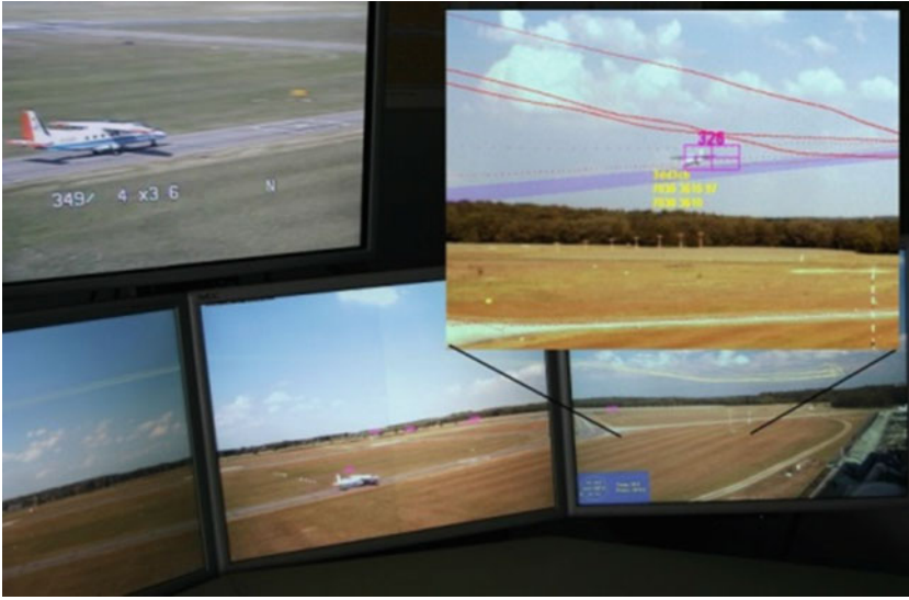
Fig. 7 Part of the initial version of the panorama display with PTZ-display on top. Inset: Screenshot of camera # 4 (=East) display showing augmentation during landing (reprinted from Schmidt et al., 2009, IEEE with permission). Superimposed glide path (violett, added for replay), GPS-trajectories (red), live multilateration position (yellow, from transponder) and automatic movement detection (red square with object number)
