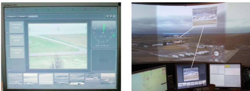
Fig. 6 Pan Tilt Zoom camera Human Machine Interface (left) and Picture in Picture (right)
