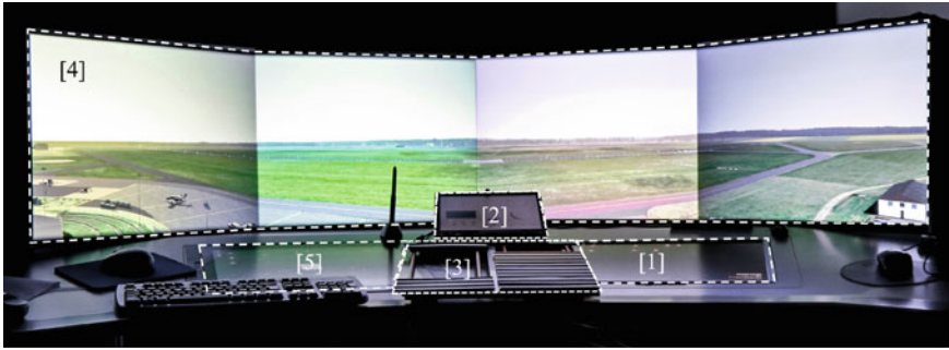
Fig. 3 Design of the RTO-CWP with [1] radar, [2] weather display, [3] flight strips, [4] far view (video panorama), [5] control display for zoom camera. The executive is positioned to the left, the coordinator to the right of the flight strips
