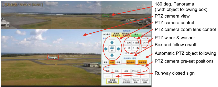
Fig. 6 Overview of the ITV display console
