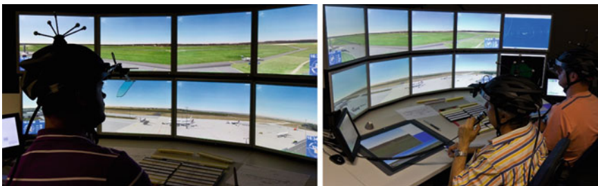
Fig. 1 Experimental remote tower center work environment for two-airport control with two video panorama systems representing the two airports, including weather information at outmost left and right displays. At the right. a (left photo) On the table flight strips are available. Operator equipped with eye-head tracking device. b (right photo): approach radar is displayed at right edge of lower panorama
