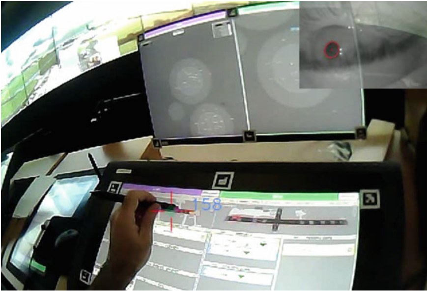
Fig. 6 ATCO's fixation and pupil dilation on the EFS and OTW with PTZ recorded by Eye Tracker to investigate HCI design and Human Performance on Multiple remote tower operations
