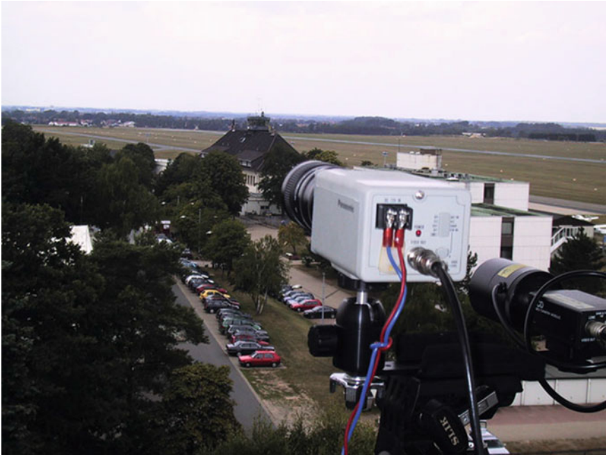
Fig. 4 Initial tests (2003) of video based far view reconstruction with standard video technology. Camera position on DLR telemetry antenna tower, ca. 25 m above ground. Camera aiming at Braunschweig airport tower on the dark roof top. White building to the right is location of initial experimental videopanorama camera system (Chap. 6). Runway visible above the camera, extending in west direction
