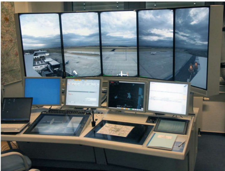
Fig. 4 Implementation of the R-CWP at Erfurt tower control room without direct airport view. Three levels of information with the video panorama in the back, the row of four flight information displays, operator console with two large touch-input displays and a small one at the right side for radio communication, are clearly structured (for details see text)
