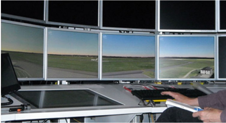
Fig. 2 Participant at a simulation console judging the outcome of a landing aircraft just after touchdown (2nd monitor from left). Approach on the rightmost monitor, touchdown is on the left side of second monitor from the right. Reconstructed panorama compressing the 180°-tower view to ca. 120° for subjects at the RTO-console (Fürstenau et al., 2012)
