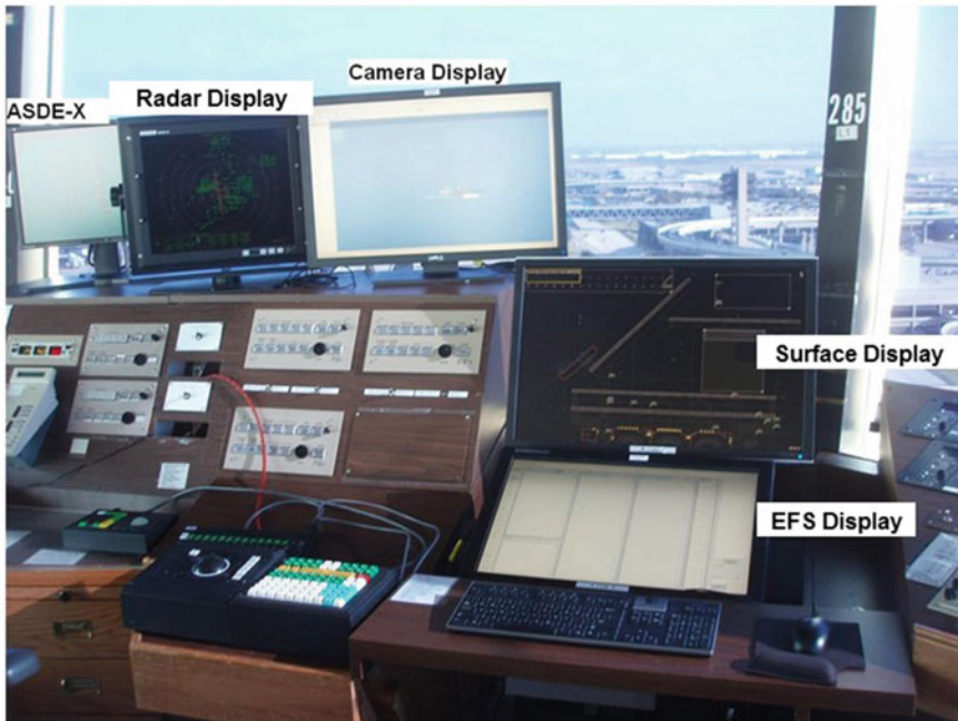
Fig. 6 DFW-2 controller workstation (Source MIT-LL)
