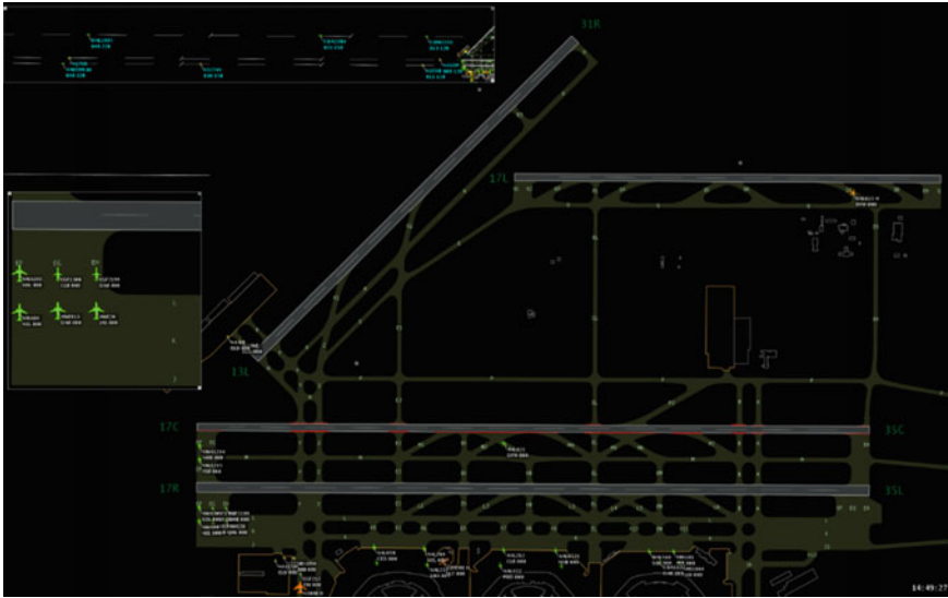
Fig. 3 Controller basic surveillance display (Source MIT-LL)
