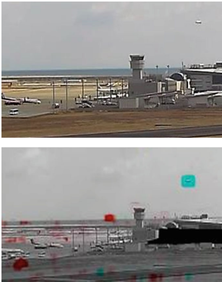
Fig. 9 Moving object detection by optical flow. The above image is a still video frame showing an aircraft on final approach and static aircraft parked on the apron the bottom image shows the optical flows: red areas indicate left-to-right and green indicate right-to-left. The approaching aircraft (moving left) has been successfully detected
