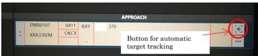
Fig. 13 Interface of electric flight strips for automatic target tracking function
