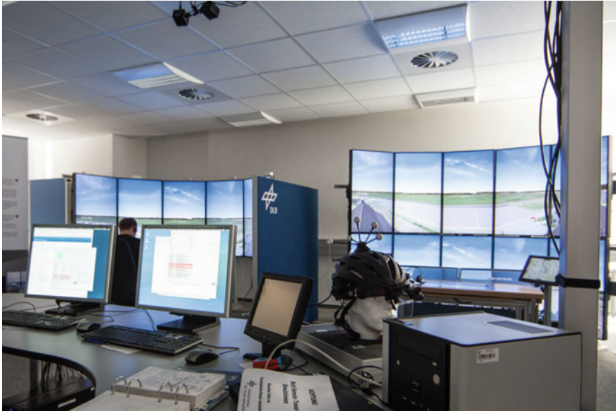
Fig. 16 Multi remote tower setup (left: single working position, right: multi remote working Position), front eye-tracking device and exercise lead working position
