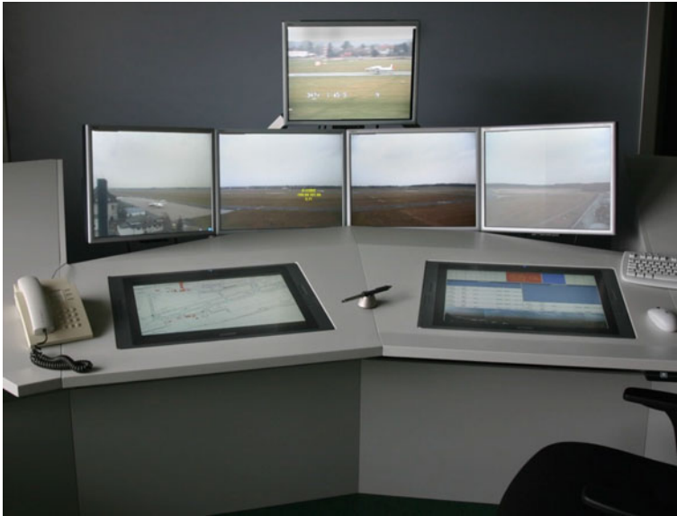
Fig. 4 Early version of 180°-videopanorama (1600 × 1200 pixel) with pan-tilt zoom camera display on top, demonstrating augmented vision function: superimposed transponder label tracking the landing aircraft using automatic movement detection (see Sect. 3.4, Fig. 7). Two pen-touch input displays integrated in the console display additional information required by the controller: the one on the right was used for electronic flight strips (flight data) and control of the camera parameters, PTZ, weather information, and tracking. Initially published in (Fürstenau et al., 2007)
