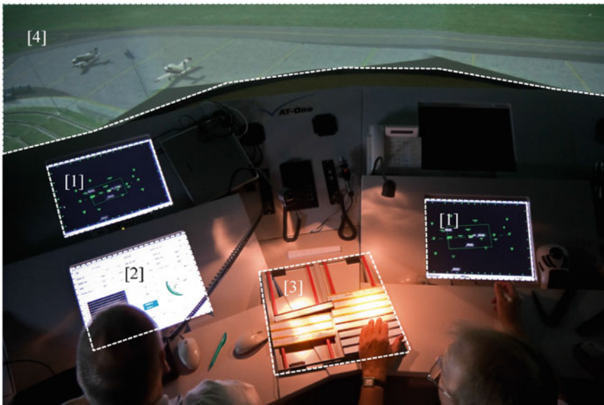
Fig. 2 Design of working positions in the tower simulator encompasses [1] two radar displays, [2] weather display, [3] flight strips; [4] far view (200° life-size projection). The executive is positioned to the left, the coordinator to the right of the flight strips
