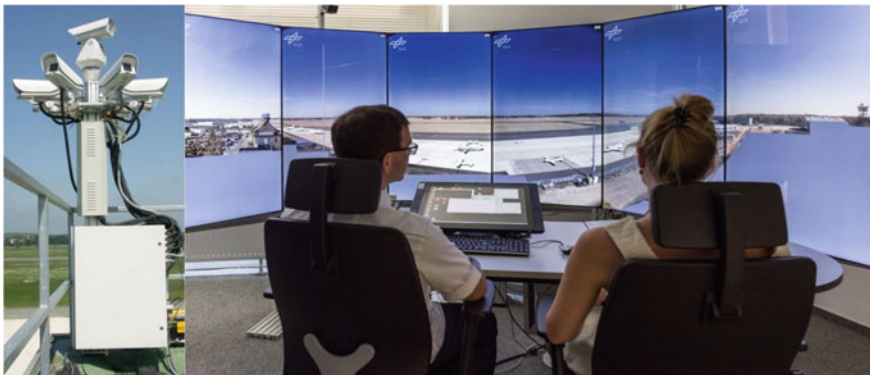
Fig. 1 DLR Remote Tower field test platform at Braunschweig-Wolfsburg Airport (BWE) (left: 360° Panorama & PTZ camera sensors; right: ATCO Participant working in passive shadow mode at the remote tower module observed and instructed by the experimenter (right))
