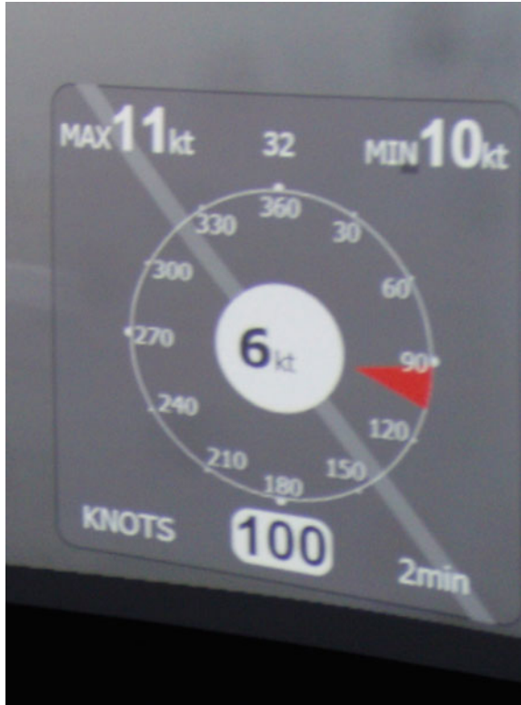
Fig. 4 Meteorological overlay with actual wind speed, direction, 2 min average and minimum–maximum values
