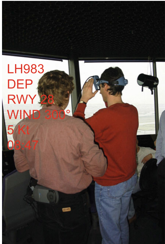
Fig. 2 Demonstration of a laser retinal scanning display, tested by controllers at Frankfurt tower under operational conditions (2/2003). Inset: Superimposed text depicts augmented vision information displayed by HMD via direct image projection onto the retina by means of a laser scanner. Wearable HMD-computing device at the back of DLR team member Markus Schmidt
