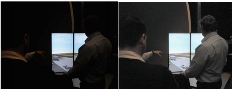
Fig. 14 Effect of decrease of display \gamma to 2.5 for increasing luminance difference in dark area while keeping contrast in high luminance display area in an acceptable range (see also Appendix A)
