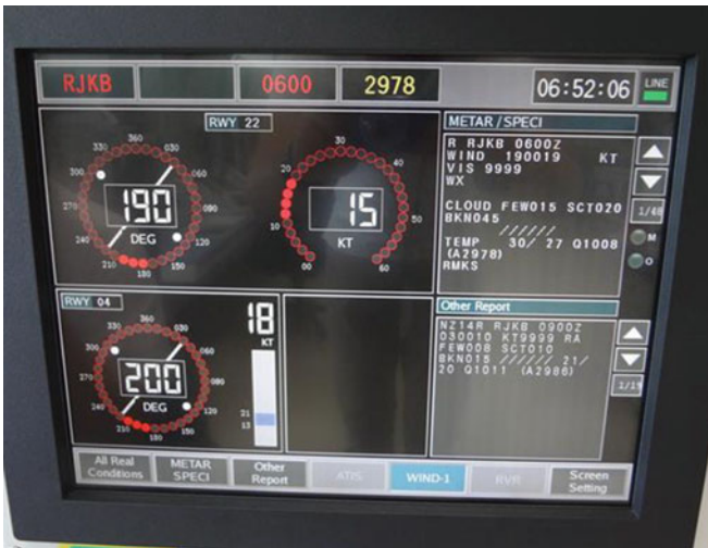
Fig. 8 TDU Display shows meteorological information data
