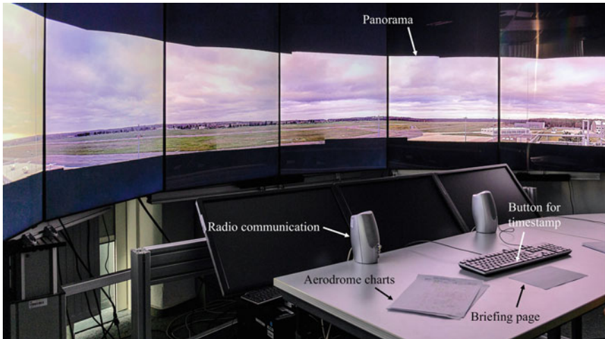
Fig. 8 Testbed in DLR's tower lab
