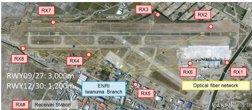
Fig. 5 Locations of the MLAT receivers at Sendai airport
