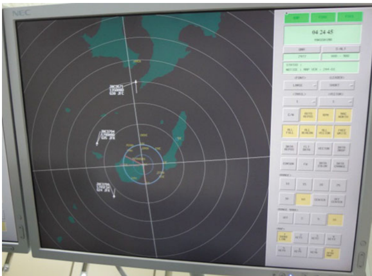
Fig. 5 APDU display shows aircraft position based on en-route radar source
