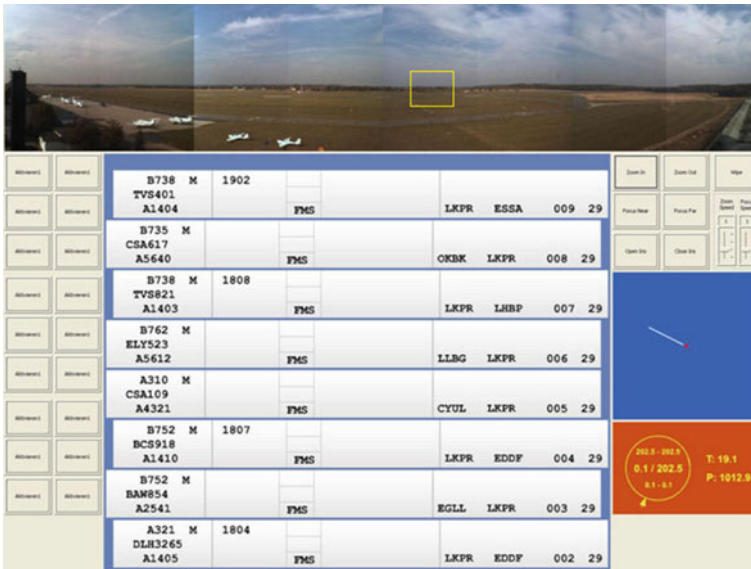
Fig. 6 Initial design of pen touch-input interaction display (reprint from: Schmidt et al., 2009), IEEE with permission). Minipanorama on top as option for PTZ positioning via touch (actual position visualized by yellow square). Center: electronic flight strips; right, from top: PTZ control buttons, virtual joystick as another option for PTZ positioning, weather data with wind direction (from weather sensors); left: optional buttons, e.g. for preset PTZ position
