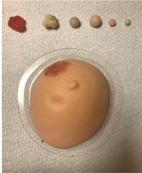
Fig. 2. Phantom breast model with 6 lumps
