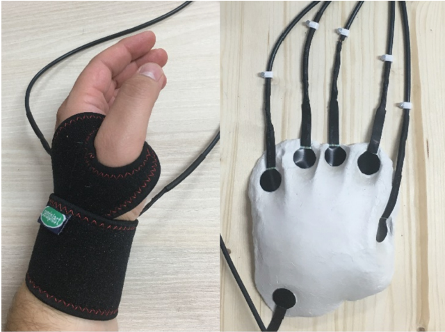
Fig. 1. Hand relaxed position/Molded part of the device with sensors
