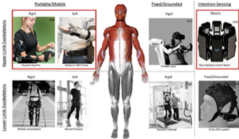
Fig. 1. Types of exoskeletons used for rehabilitation and new intention-sensing technologies [11]
