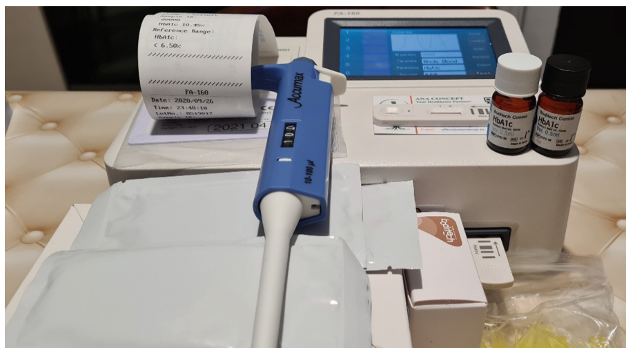
Fig. 3. The experimental setup containing the FA-160 immunofluorescence analyzer and the testing materials.
