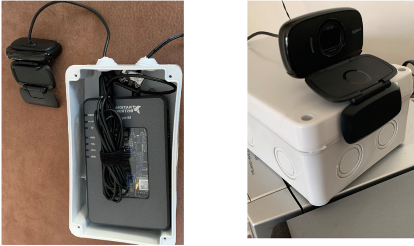
Fig. 3. MyRIO based image acquisition unit and its housing
