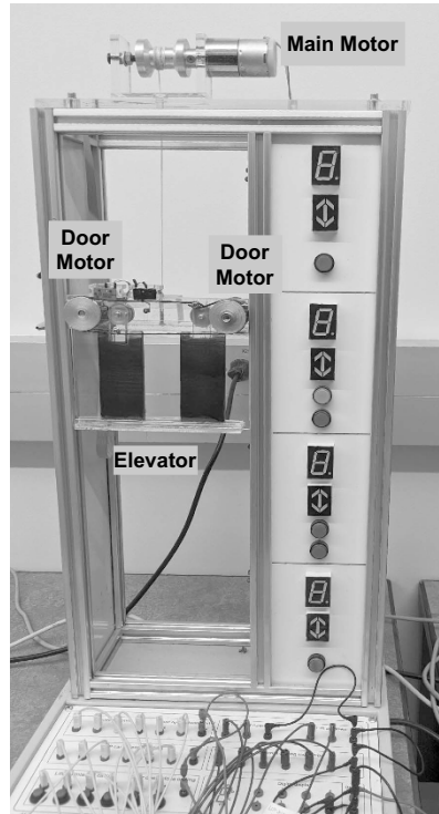
Figure 9. Front view of the elevator testbed.
