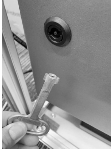
Figure 2. Control box lock and key.
