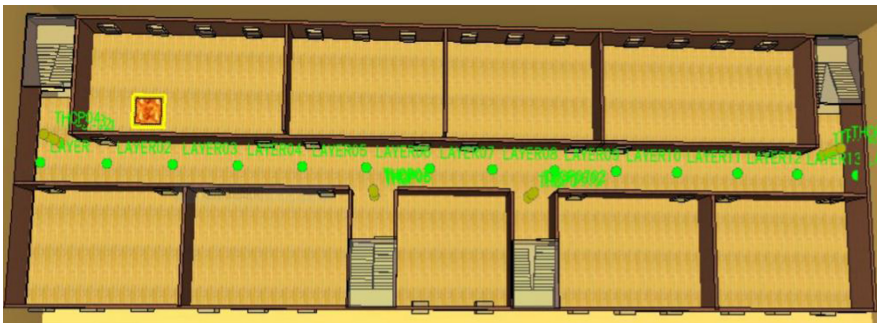
Fig. 4. The setting of thermocouples
