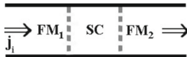
Fig. 19.2 Illustration of a magnetic tunnel junction consisting of two ferromagnetic metals ( FM ) 1 and ( FM ) 2 separated by a superconductor (SC). The electron current j_e , as well as j_\uparrow and j_\downarrow and j_s = j_\uparrow - j_\downarrow , depend on the relative orientation of the magnetisations \vec{M}_1 and \vec{M}_2 and on the superconducting state, singlet vs. triplet Cooper pairs. Note, M_2 - M_1 = \Delta M may cause Josephson-like spin current, which is particularly affected in the case of a triplet superconductor by the phase of its order parameter. Of course, the spin current is destructively affected by spin flip scattering
