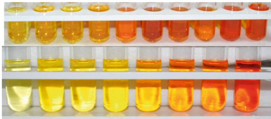
Fig. 3.4 CdSe core QDs synthesized at 160 °C with Cd:Se ratio of 1:10 are shown under ambient light
