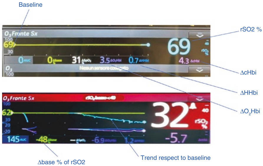
Fig. 26.3 Near infrared spectroscopy. This figure represents two possible traces, one with normal values and the other with abrupt decrease in regional oxygen saturation ( rSO_2 ) values. \Delta O_2Hbi index associated with variation of the oxygenated component of the hemoglobin in the total calculation of rSO_2 (arterial component of rSO_2 ), \Delta HHbi an index associated with variation of the deoxygenated component of hemoglobin within the total calculation of rSO_2 (venous component of rSO_2 ), \Delta cHbi is the sum of \Delta HHbi + \Delta O_2Hbi . SpO_2 - rSO_2 is the difference between the value of peripheral saturation of oxygen ( SpO_2 ) and rSO_2
