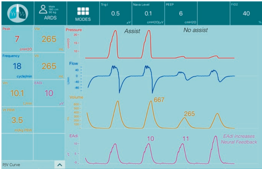
Fig. 7.3 This figure illustrates the comparison of neuro ventilatory efficiency (NVE = V_T/EAdi ) between one assisted breath ( NVE_{\text{assist}} = 667/10 = 66.7 \text{ mL}/\mu\text{V} ) and one unassisted ( NVE_{\text{unassist}} = 265/11 = 24 \text{ mL}/\mu\text{V} ). Patient Ventilator Breath Contribution = 100 \times 24/66.7 = 36\% . (Figure comes from the application iVentilate. Courtesy of Pr Hadrien Rozé)
