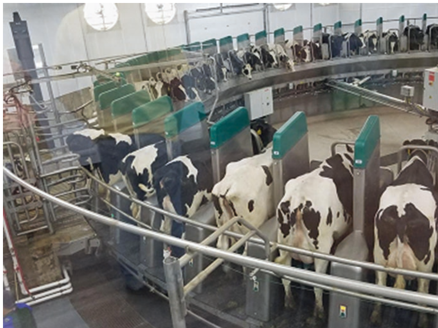
Fig. 11.24 The robotic rotary milking parlor. (Source: https://www.agupdate.com/farmandranch-guide/news/dairy/new-robotic-milking-parlor-features-the-latest-in-technology/article_eb6e9530-9826-11e8-ad4a-8329f5374a69.html )
