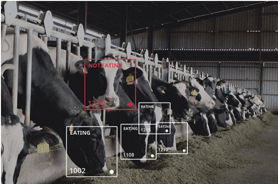
Fig. 11.21 Intelligent computer vision for identifying each cow in the herd and monitoring its daily habits. (Source: https://www.cainthus.com/ )
