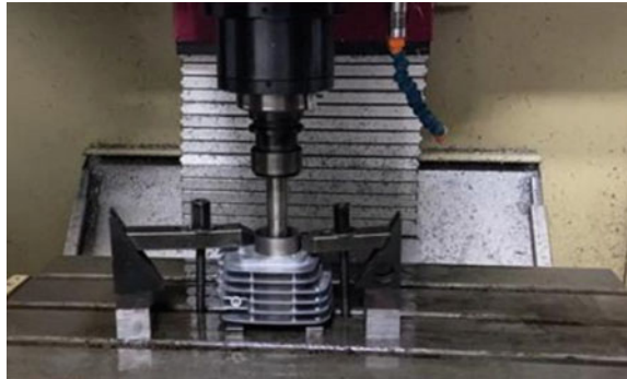
Fig. 18.8 Set up specimens and set all axes to zero
