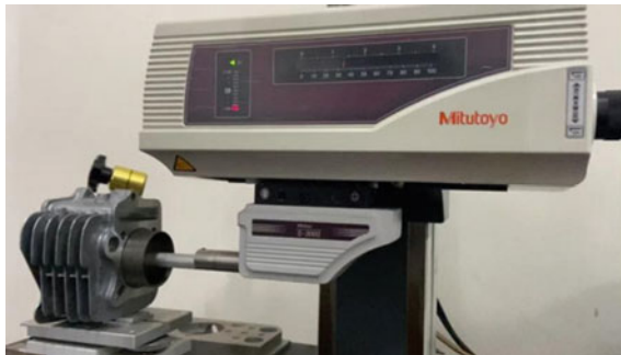
Fig. 18.5 Tested surface roughness started
