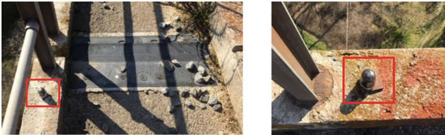
Fig. 2 Wireless accelerometers mounted on the side walkway (10 g full-scale)
