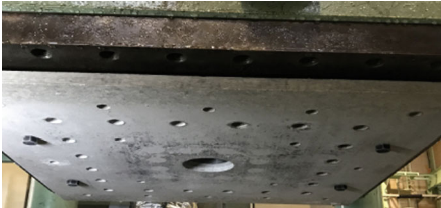
Fig. 4 Insulation plate (on the upper surface of specimen)
