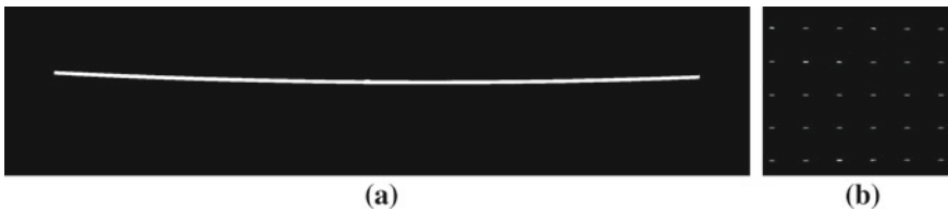
Fig. 6 Image segmentation; a still frame of cable specimen; b segmented image into 30 equal parts
