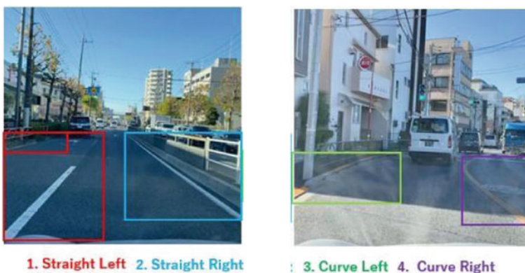
Fig. 7 Four classes for road lane line detection
