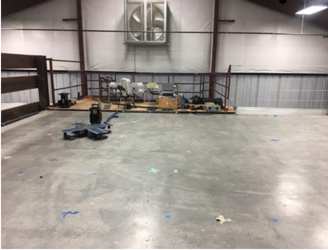
Fig. 2 The MTMD placed at the quarter point of the test floor
