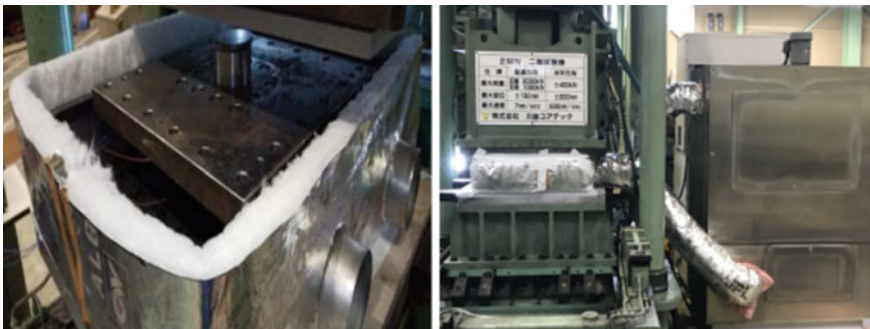
Fig. 3 Insulating chamber (left) and cooling system (right)
