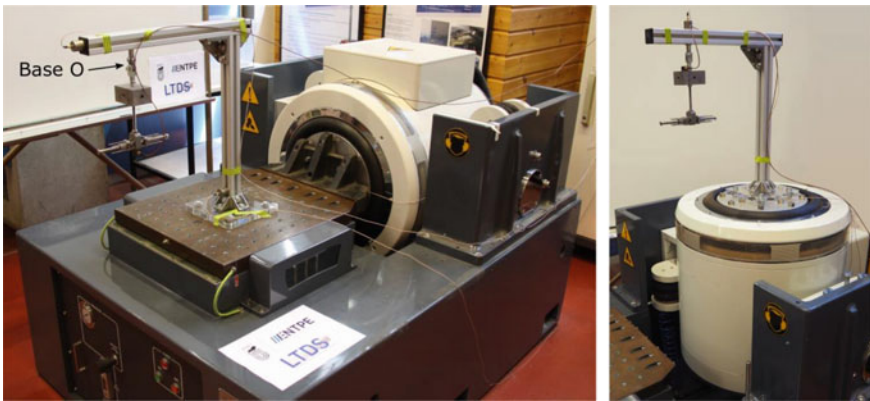
Fig. 5 Reduced model on the shake table in horizontal and vertical position [8]
