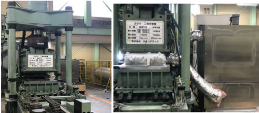
Fig. 5 200tf loading system (left) and cooling system (right)
