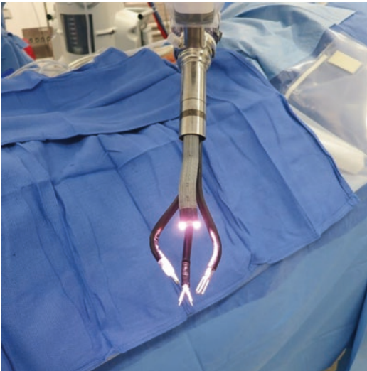
Fig. 21.3 The double joint feature of the SP camera and instruments
