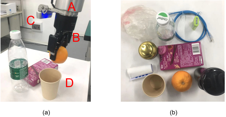
Fig. 4. Experiment setup. (a) Robot experiment on a cluttered scene. A: UR-10e Robot; B: Robotiq two-finger parallel gripper; C: Intel RealSense RGBD camera; D: Graspable objects. (b) Household objects for the experiment.
