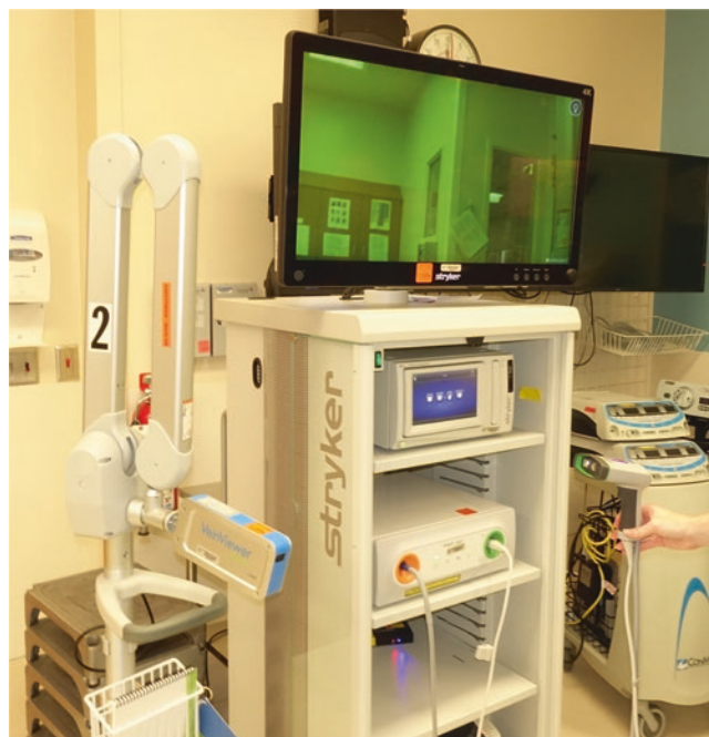
Fig. 5.4 Commercial devices for indocyanine green (ICG) fluorescent lymphography include the PhotoDynamic Eye (PDE, Hamamatsu Inc., Japan) and the SPY Phi (Stryker Inc., USA) (right). For surgical planning, the adjunctive use of a vein imager can aid in identification of nearby venules and assessment of their valvular competence for selection for anastomosis (left)
