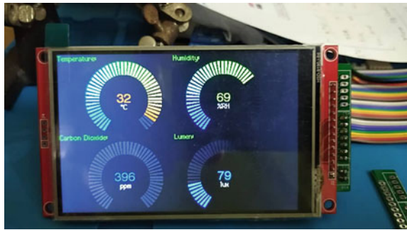
Fig. 12.7 System for environmental condition monitoring oyster mushroom indoor cultivation
