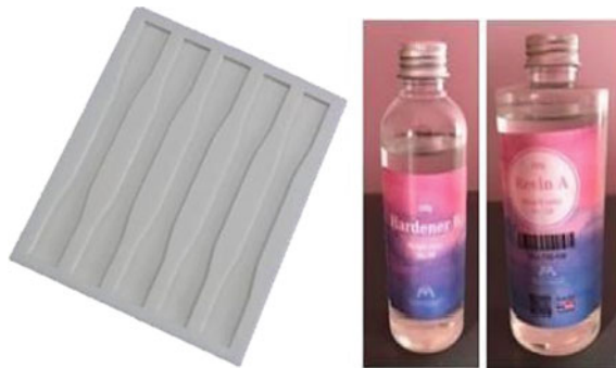
Fig. 1.1 Silicone rubber mold (SRM), hardener, and epoxy resin
