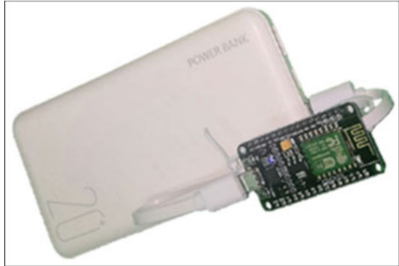
Fig. 26.1 Parental device of the proposed monitoring system
