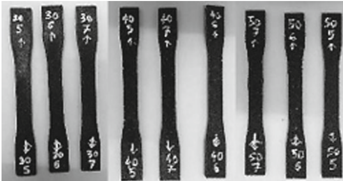
Fig. 1.4 Dumbbell tensile test specimen ASTM D638-14
