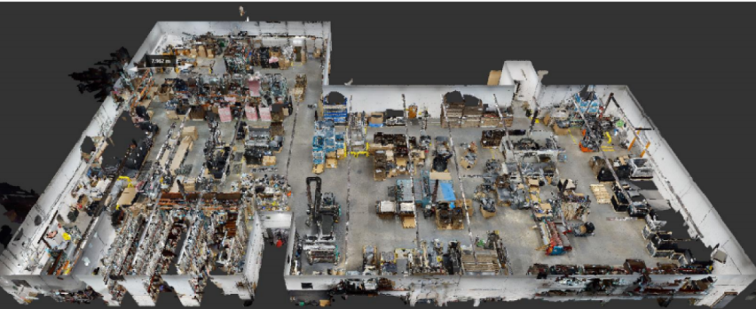
Fig. 2. Areal view of the shopfloor with 3D scanning photogrammetry (a) and structure light (b) type
