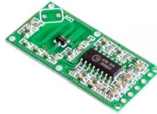
Fig. 2. Microwave radar sensors based on the Doppler effect
