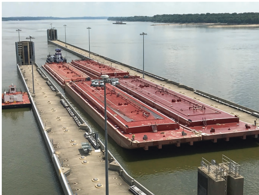
Fig. 10.9 Typical four-barge tow at Olmsted Lock and Dam, Liquid Bulk, Ohio River. (Courtesy of US Army Corps of Engineers, Louisville District)
