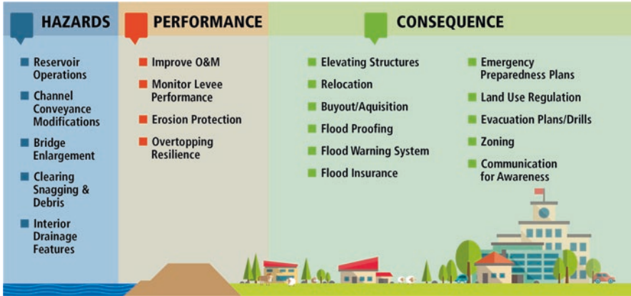
Fig. 14.11 Example risk management measures to address the different components of risk. (O&M stands for operation and maintenance activities)
