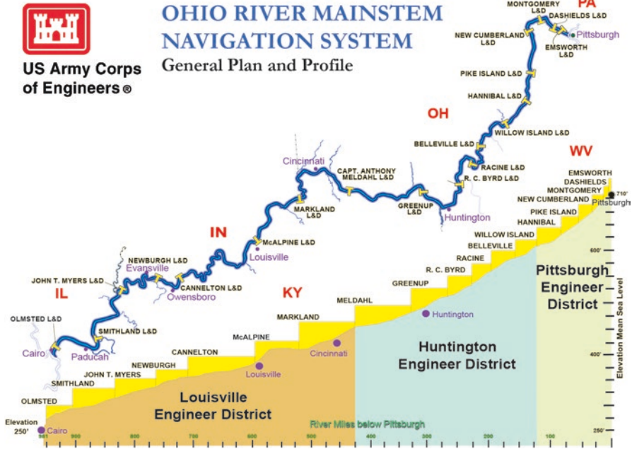
Fig. 10.5 General plan and profile of the Ohio River. (Courtesy of US Army Corps of Engineers, Louisville District)
