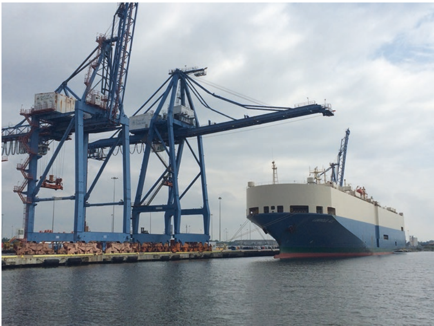
Fig. 11.2 The vehicle carrier vessel Luminous Ace awaits cargo at the Port of Baltimore. Economies of scale and shipping alliances have hastened the production of massive vessels. As of 2020, the Port of Baltimore is expanding terminals and deepening its berths to accommodate Neopanamax vessel sizes. (Photo courtesy of Katherine Chambers)
