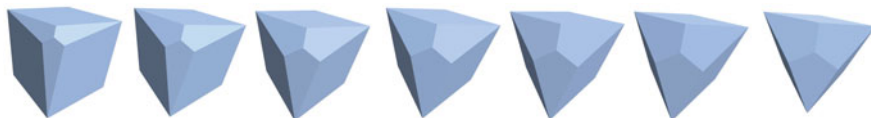
Fig. 16 Adjusting the depth of the slanted cut through a vertex, varying from a cube to a Sharpohedron to a tetrahedron
