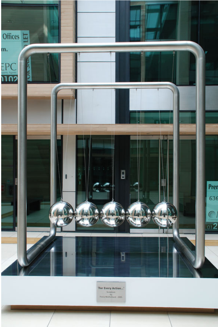
Fig. 2 In the standard textbook description of Newton's Cradle there is always only one sphere in motion. However, careful observation of the experiment shows that, already after the first impact of a displaced sphere on one side, the entire chain begins to break up, with all spheres in motion. Theory and computer simulations confirm this, and attribute it to the finite elastic modulus of the spheres [7]. The photograph shows the stainless-steel sculpture For every action ... (2005) by Fiona Mulholland permanently sited at Beacon Court South Quarter, Sandyford, Co Dublin. (Photo reproduced with kind permission by the artist)
