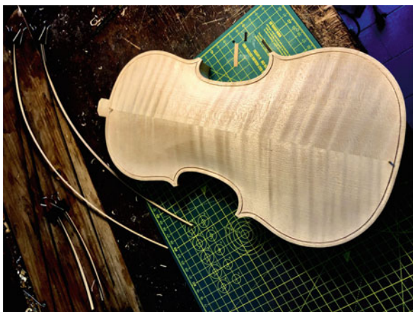
Fig. 12 Excavation of the purfling's channel; courtesy of luthier Federico Mari
