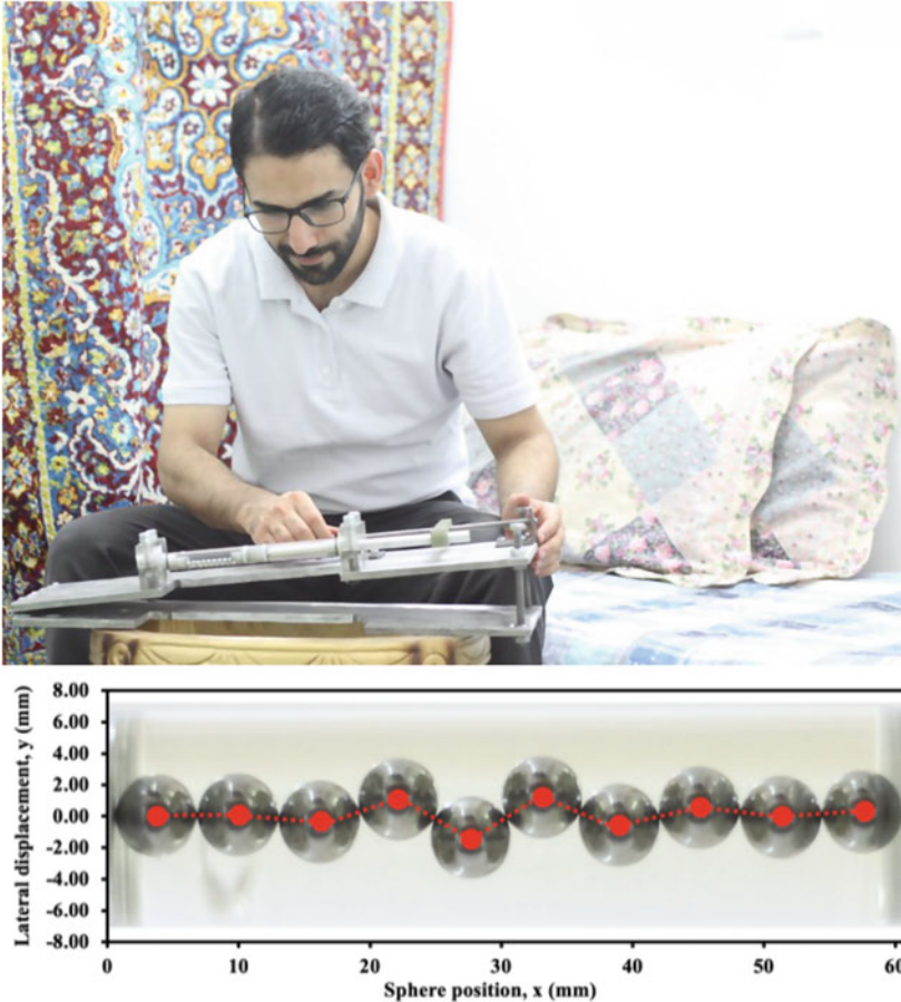
Fig. 1 One of the authors (AI) performing experiments in his bedroom in Tehran, Iran, during a Covid lock-down. His apparatus consists of a cylinder containing metal spheres. Pushing in the sides of the cylinder induces buckling of the initially linear chain. The effect becomes more and more localized as the compression is increased. In a variation of the experiment we study the position of the localisation peak as the cylinder is tilted, in order to determine the so-called Peierls-Nabarro potential [4]. This potential, originating in the theory of crystal dislocations, can tell us how the localized buckling moves when we tilt the apparatus
