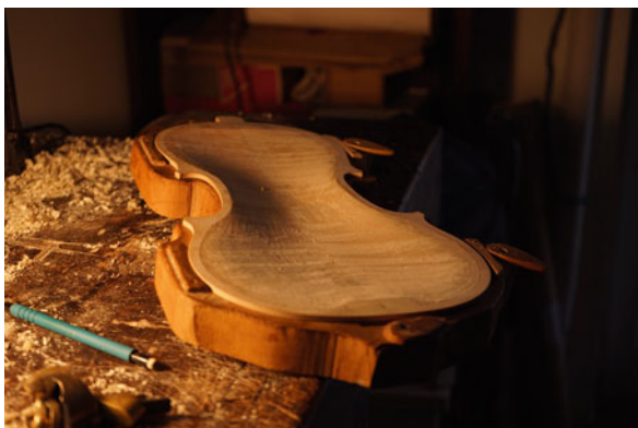
Fig. 14 Intermediate phase of the internal sculpture of the bottom; courtesy of luthier Federico Mari
