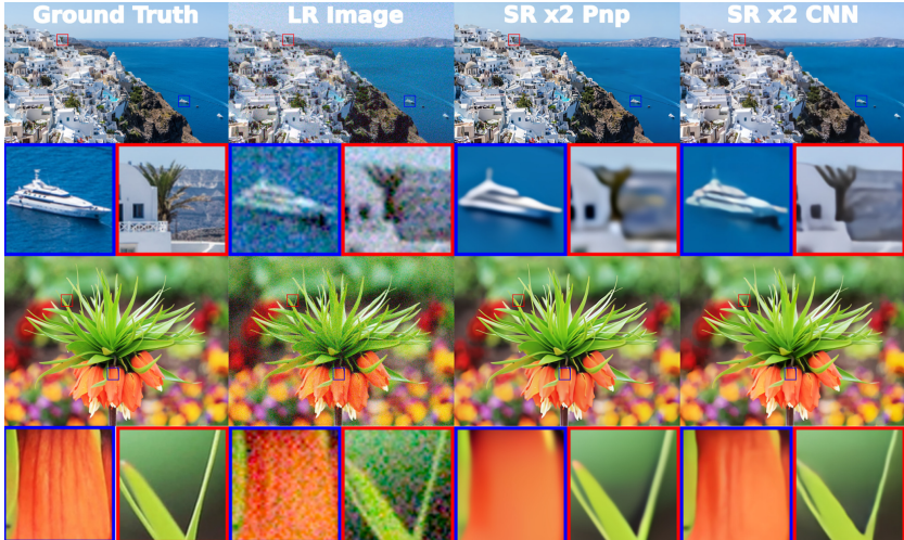
Fig. 5. Qualitative comparison of super-resolved images produced by the PnP approach with the L_1 -trained CNN (spatial variation). The results from the CNN have sharper details and more realistic textures.
