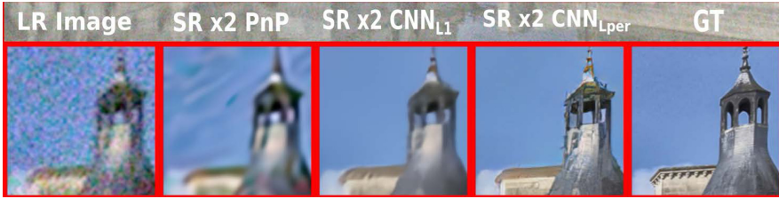
Fig. 4. Visual examples of the noise experiment on one of the test images degraded with the varying blur kernels shown in Fig. 1 (left) and realistic noise with noise levels given by a = 0.011, b = 0.0001 .
