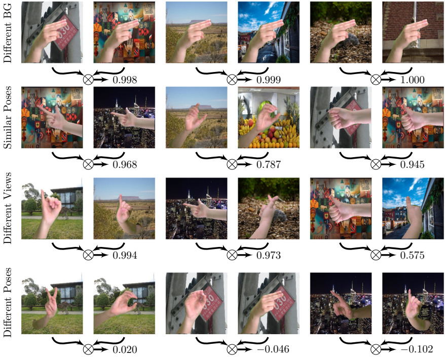
Fig. 3. Examples showing the cosine-similarity scores for the embeddings produced by pretraining. The first row shows embeddings for the same hand pose with different backgrounds, the embedding learns to focus on the hand and ignore the background. In the second row we show images for similar hand poses, with different background, these also score highly. In the third row different hand poses, with the same background produce low scores.
