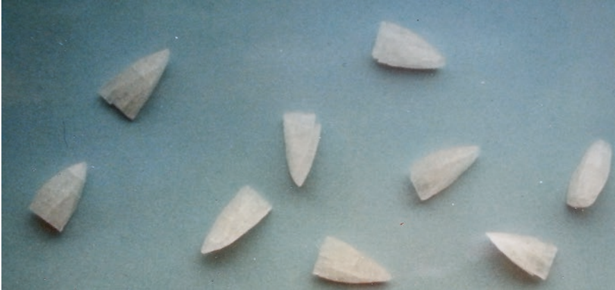
Fig. 1.1 Single crystals of \alpha -lactose monohydrate produced by growing them individually in aqueous lactose solutions of constant supersaturation and used in single crystal experiments (Jelen 1972; weight of the crystals approx. 0.25 g, length about 1.5 cm)
