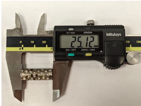
Fig. 1 4 mm steel-steel composite metal foam (S-S CMF) prepared for coefficient of thermal expansion measurements
