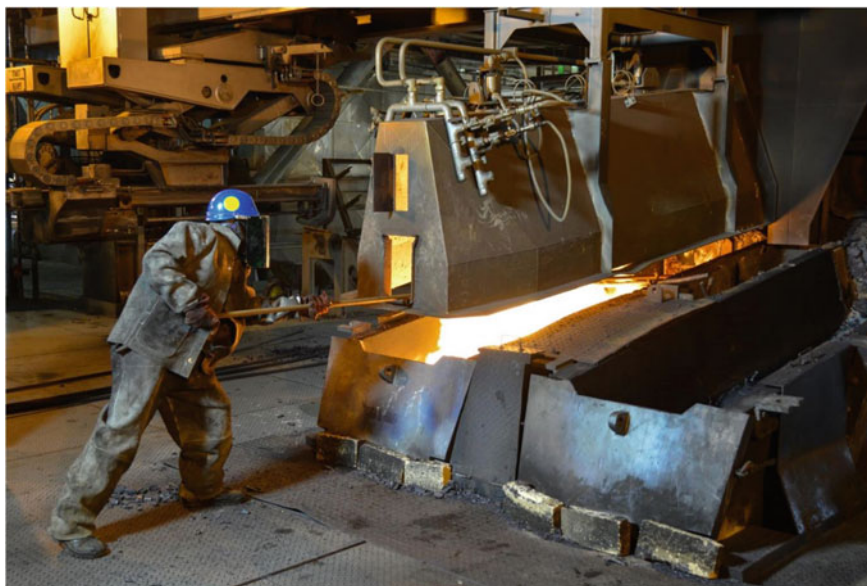
Fig. 2 Multi-phase tapping of an ISASMELT™ furnace
