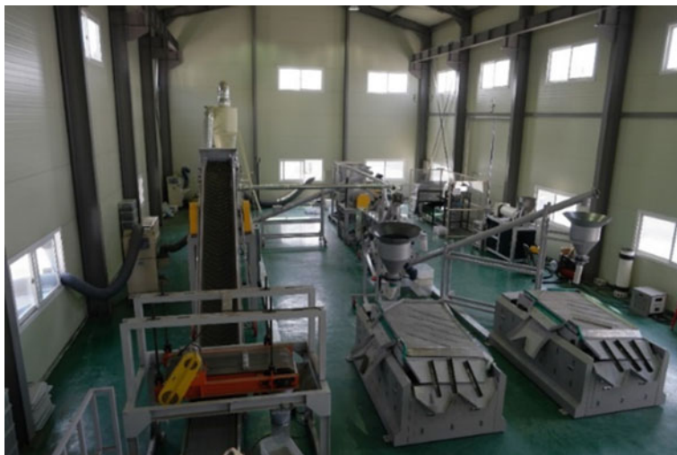
Fig. 9 Photograph of physical separation facility for ASR recycling of ELVs
