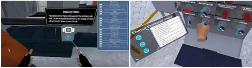
Fig. 7 Interactive checklist guides users through orientation where they learn about the die casting machine (left). A startup procedure sheet guides users through the step-by-step process of safety and status checks and control sequences to turn on the die casting machine and begin producing parts (right)
