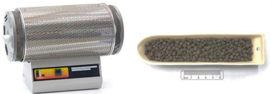
Fig. 7 Tube furnace at the Chair of Nonferrous Metallurgy, Montanuniversität Leoben (left) and ceramic shuttle with micro-pellets (right)
