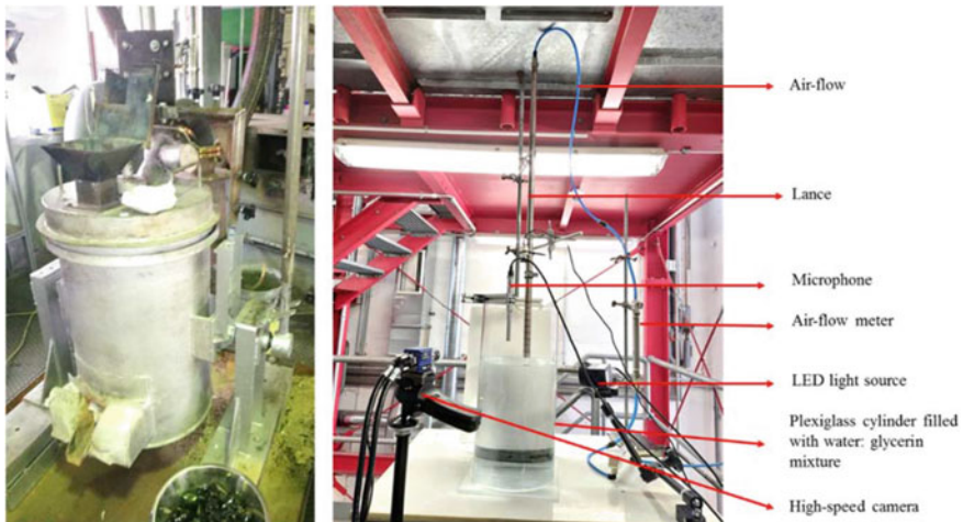
Fig. 2 Left: Laboratory/small-scale TSL smelter at the Institute of Nonferrous Metallurgy and Purest Materials (INEMET), TU Bergakademie Freiberg. Right: Geometrically similar TSL cold model set-up
