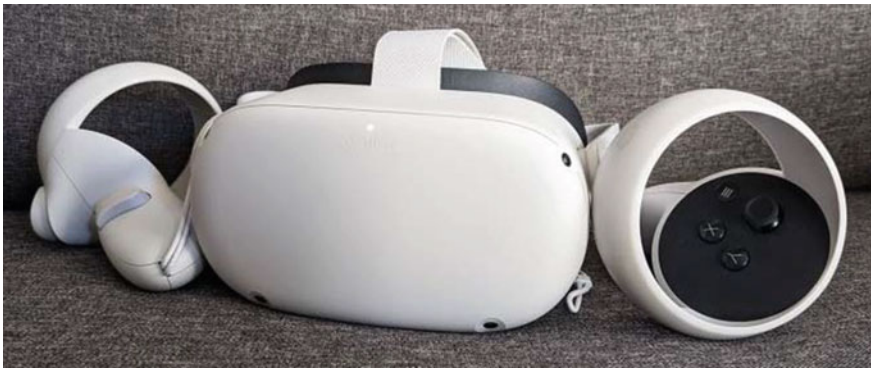
Fig. 3 Oculus Quest 2 VR system enables users to view the virtual environment on a tracked 3D headset and interact with the environment using two tracked 6-DOF controllers
