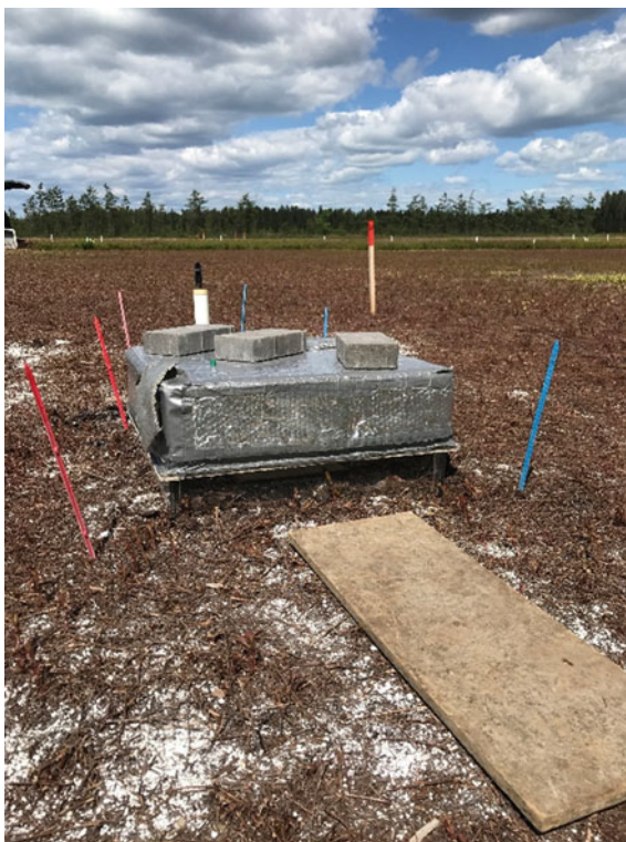
Fig. 2 Non-flow-through, non-steady chamber for the greenhouse gas emission monitoring
