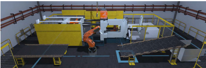
Fig. 1 Virtual die casting machine, and surrounding environment was modeled based on configurations used in industry, including die casting cell layout, safety guards, and support equipment
