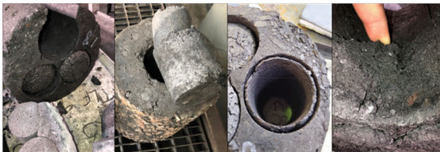
Fig. 7 Pictures showing results of the Elkem baking “Drop” test and the performance of the Eltap™ G THL
