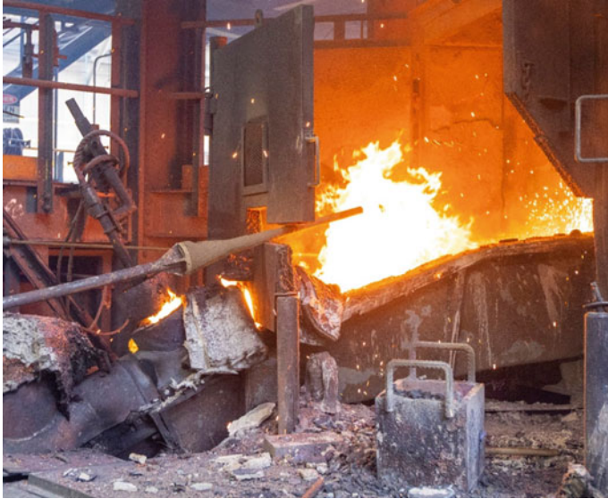
Fig. 4 An MPP just before closing a blister tap-hole
