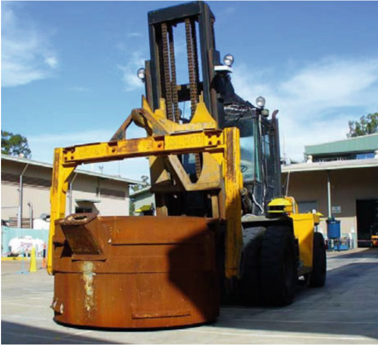
Fig. 4 AGV Hot Metal Carrier in the process of picking up a small crucible. Source CSIRO
