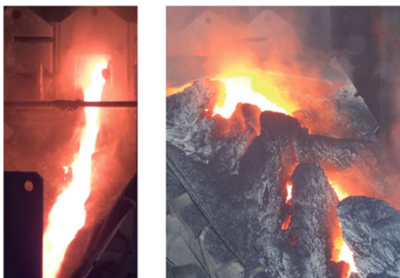
Fig. 13 Freeze lining in lead ISASMELT™ tapping launder at Kazzinc Ltd.
