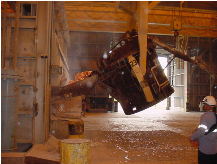
Fig. 5 Crucible emptying into a furnace using a crane and a feeding trough
