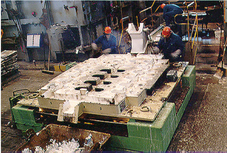
Fig. 14 Flooded table direct chill extrusion billet casting
