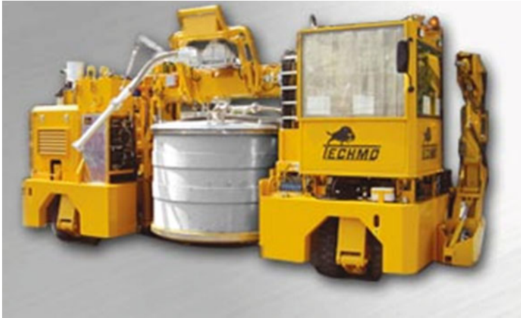
Fig. 8 Pressurised crucible transport system
