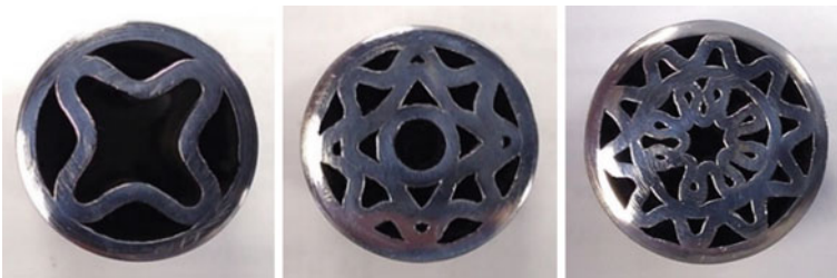
Fig. 4 Different thermal lance profiles used in the examples of this document. Model 1: SOB 38 (3/8 in.) (left), model 2: TR-38 (3/8 in.) (center) and model 3: TR-50 (1/2 in.) (right). Lance model 2, have a unitary mass per length of 1.23 kg/m and a total required oxygen inlet flow of 58.26 Nm 3 /h
