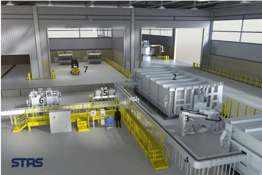
Fig. 9 General cast house layout. Ladle treatment at 1. Furnaces at 2 receive metal from the cells. At 3 is the rotary flux injector. The launders (4) transport metal from the furnaces. Metal flows to the inline degasser (5) and then the filter (6) along the trough and finally to the casting machine (not shown on left). Skimmed dross goes to the dross coolers (7). Source STAS
