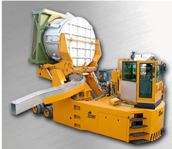
Fig. 6 Combined crucible tilter and transport vehicle
