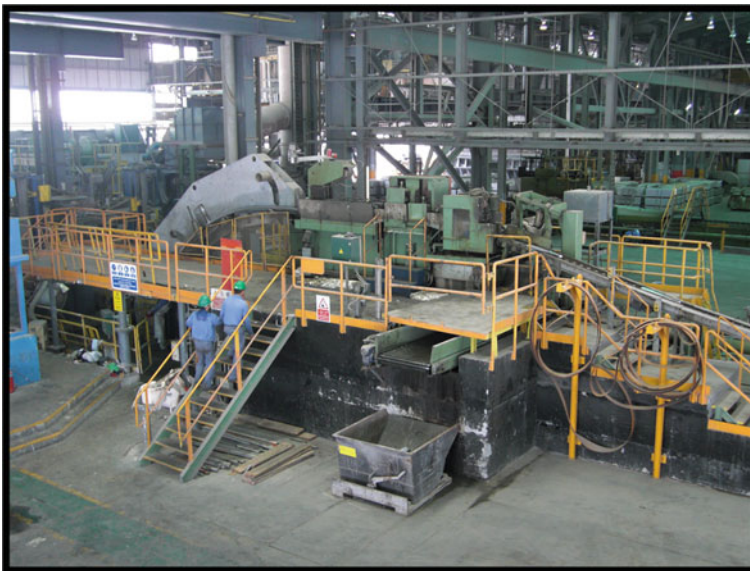
Fig. 17 Large wheel and belt caster for casting of 10 kg remelt ingots. Source Aluminium Bahrain
