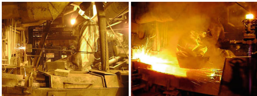
Fig. 6 Lance ignition (left), lancing operation (right)
