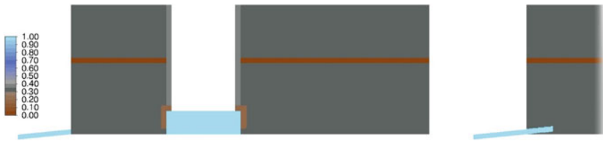
Fig. 3 Porosity distribution in idealized Si-furnace (left) and an alternative distribution with extended tap-hole (right)
