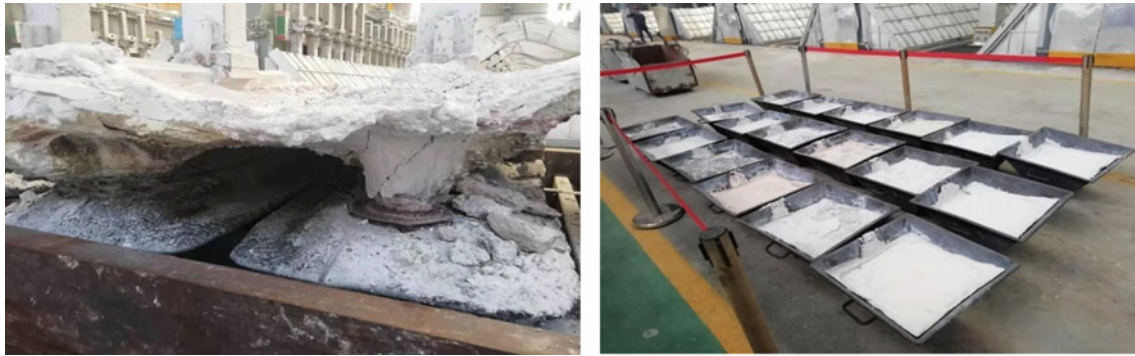
Fig. 3 Characteristics of Hot Cell: anode stubs were washed by electrolyte melt and large amounts of electrolyte melt were removed from the 18 cells
