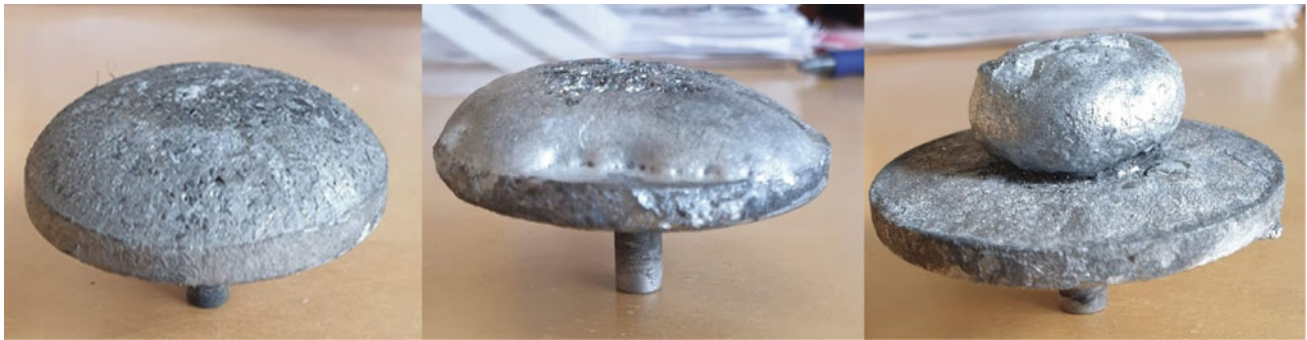
Fig. 6 Deposits obtained at T = 965 °C for a blank test to the left, 3 wt.% Mn initially in the bath in the center, and 1 wt.% Si to the right
