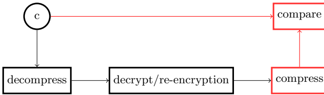
Fig. 1. Visualisation of the FO-transforms re-encryption check including decompression and compression. Being able to introduce one-bit faults anywhere in the red (light) phases enables our attack. (Color figure online)
