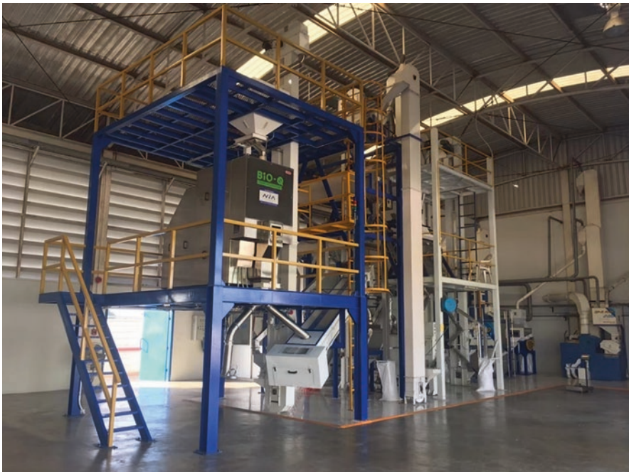
Fig. 28.3 Commercial BIO-Q RF technology machine controlling rice weevil in milled rice
