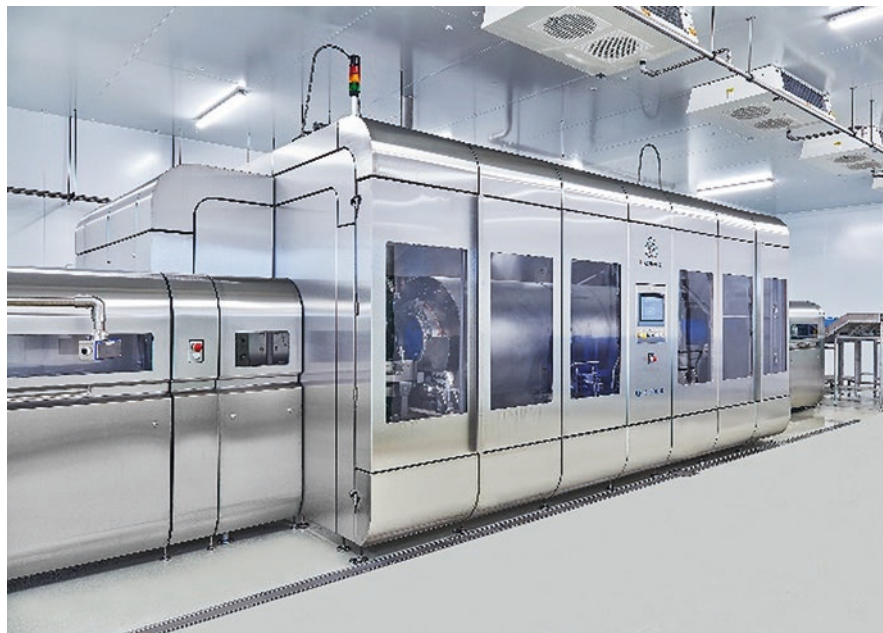
Fig. 15.2 HHP Uhde 350–60. (Source: Uhde High Pressure Technologies GmbH, HPP Center Quakenbrück, Germany)
