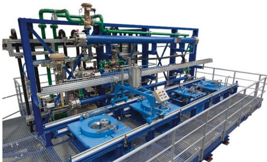
Fig. 15.3 2×200L Supercritical Extraction Plant, USA, with permission of Uhde GmbH
