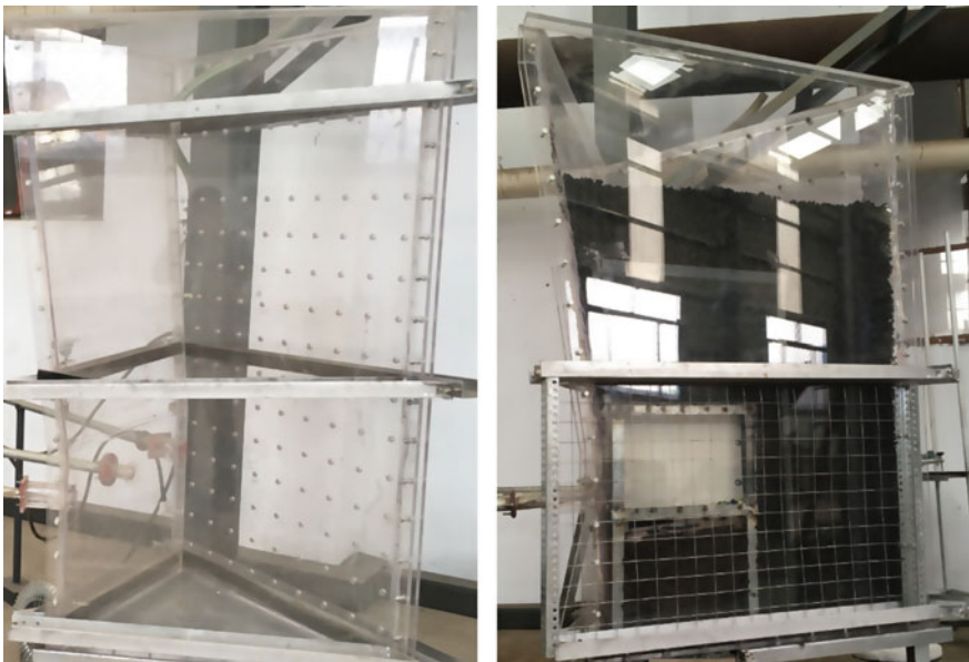
Fig. 1 3D model experimental facility (empty and charged)
