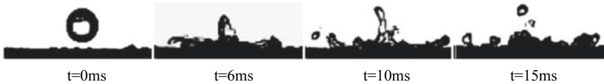
Fig. 5 Droplet impact behavior on the tailings surface in splash with continuous liquid film regime. T_s = 450\text{ }^\circ\text{C} We = 67.6
