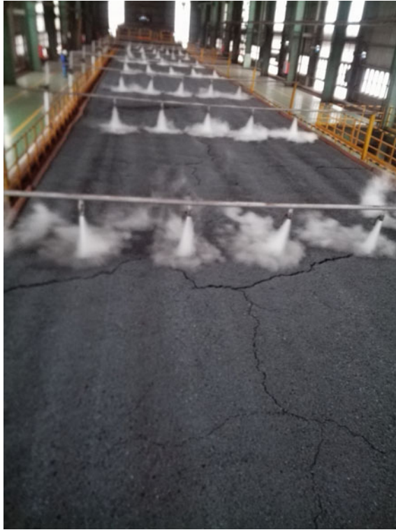
Fig. 1 Schematic diagram of steam injection on sinter surface in Jingtang
