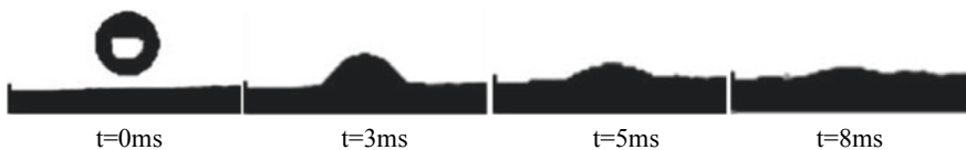
Fig. 2 Droplet impact behavior on the tailings surface in spread regime. T_s = 200 °C We = 42.8
