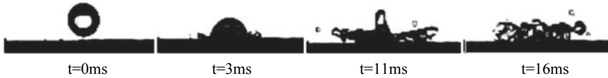
Fig. 3 Droplet impact behavior on the tailings surface in boiling induced break-up regime. T_s = 300\text{ }^\circ\text{C} We = 31.7
