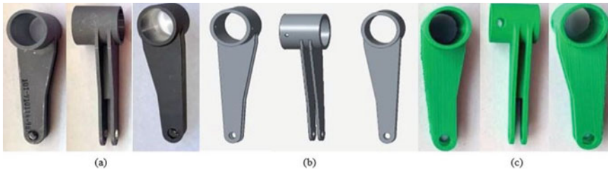
Fig. 2 Reverse engineering process: a obsolete physical part, b CAD model of obsolete part, and c pattern for sand casting of the reversed part using material extrusion additive manufacturing
