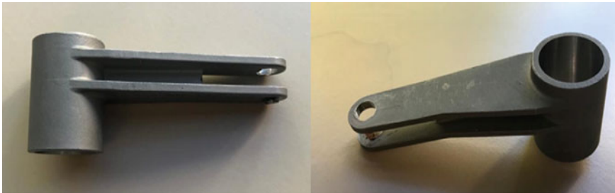
Fig. 4 Final reverse-engineered part using sand casting from 3D printed pattern
