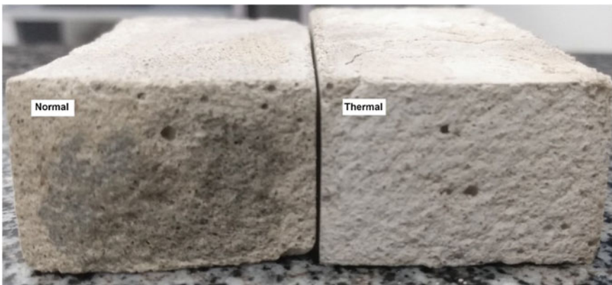
Fig. 5 Illustration of geopolymer tile specimens with 20% FGD
