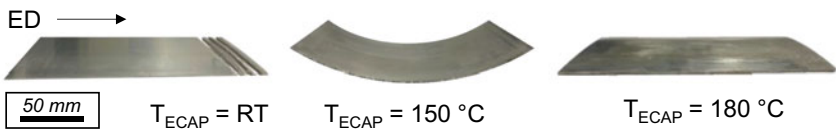
Fig. 3 ECAP specimens after one pass at different processing temperatures with a channel angle of 110^{\circ}
