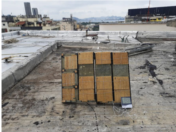
Fig. 2 Sample holder apparatus placed on the roof of a building in Rio de Janeiro/Brazil
