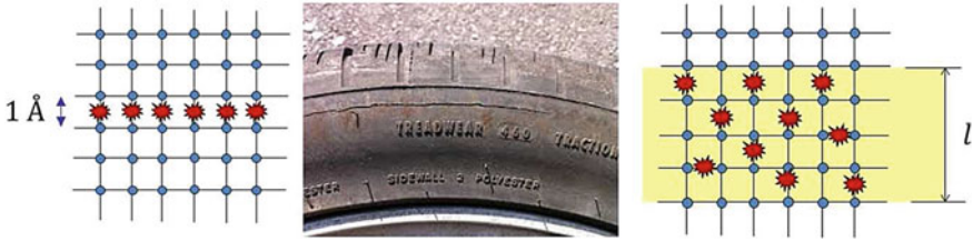
Fig. 8 Left: idealized crack with zero thickness; center: visible closed crack in unloaded tire; right: realistic bulk crack with finite thickness l
