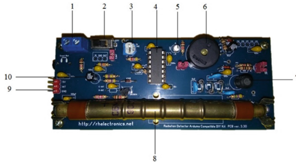
Fig. 3. Radiation detector compatible with Arduino Uno
