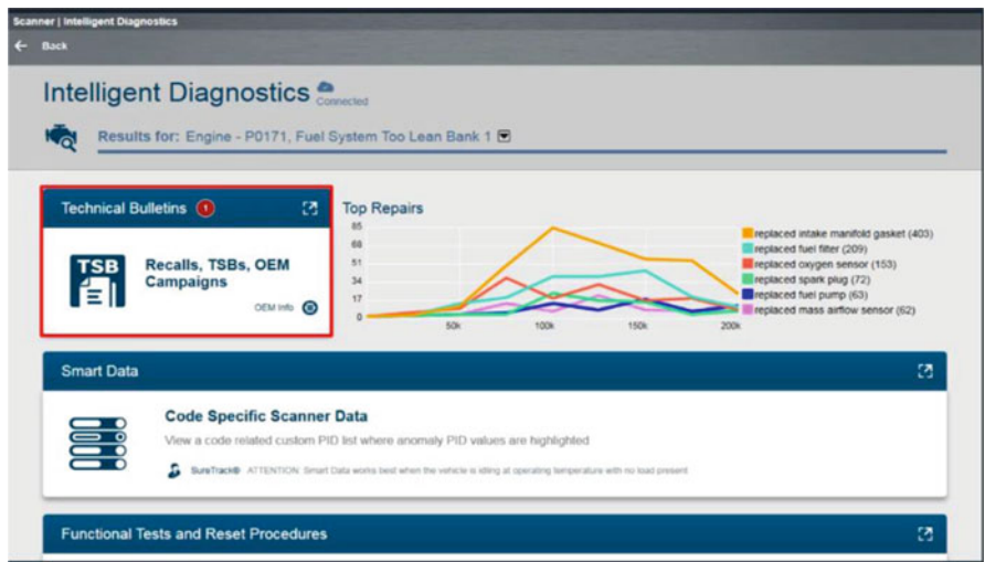
Fig. 1.3 Predii’s intelligent diagnostics interface for analyzing repair order data
