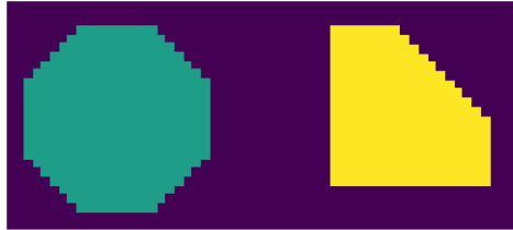
(b) The achieved propagation shown for two pedestrians. The left one with 1 meter/sec omnidirectionally and the right one with 2.7 meters/sec limited to the directions {0, 6, 7}.
