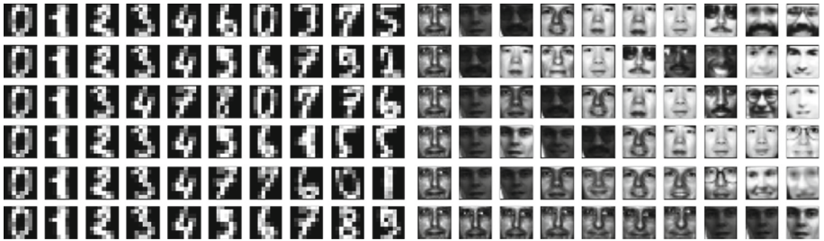
Fig. 3. Comparison of prototypes using the squared euclidean, euclidean, cityblock, minkowski, cosine and hamming distances obtained from GES and DaC algorithms. Hamming distance provides the most meaningful prototypes in MNIST, that is explained by the nature of the data as data images are really sparse and the fact that hamming distance calculates the number of the different entries in the data. Minkowski distance identifies few types of number 5, euclidean distance identifies all the classes apart from class 8. In Faces dataset, on contrary, the most meaningful prototypes are provided by euclidean, squared euclidean, cityblock and minkowski distances, allowing to have a variety of prototypes to preview a dataset.
