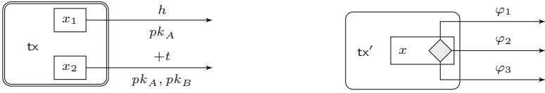
Fig. 1. (Left) tx is published on the blockchain. The output of value x_1 can be spent by a transaction containing a preimage of h and signed w.r.t. pk_A . The output of value x_2 can be spent by a transaction signed w.r.t. pk_A and pk_B but only if at least t rounds passed since tx was accepted by the blockchain. (Right) tx' is not published yet. Its only output can be spent by a transaction whose witness satisfies \varphi_1 \vee \varphi_2 \vee \varphi_3 .
