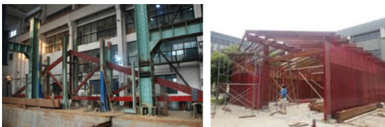
Fig. 12 Large span GluBam truss
