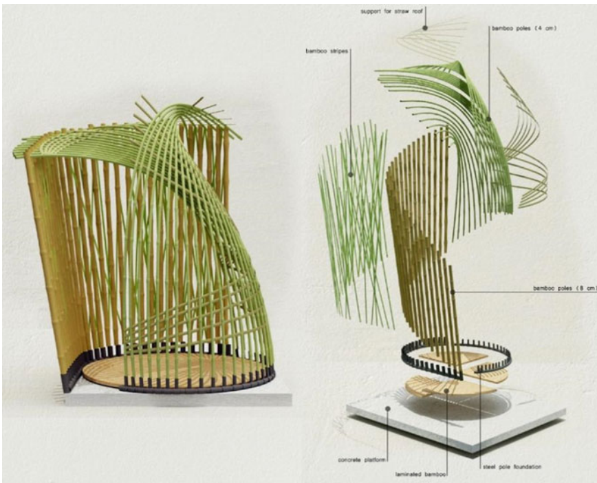
Fig. 9 Artistic representation of the structure and exploded view of the structural elements
