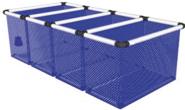
Fig. 5.11 Sketch of floating cage using in seaweed cultivation (Kasim and Mustafa 2017)
