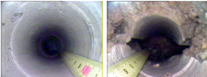
Fig. 7. Boroscopy images. (Left) solid stone material (right) rubble stone material
