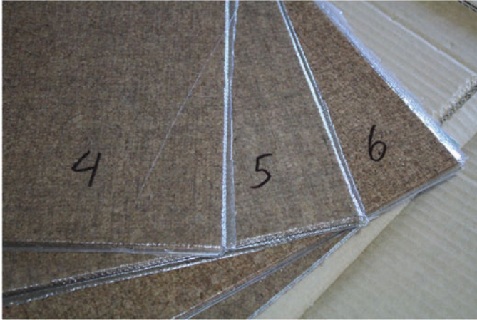
Fig. 5.1 Flax fibers laminates with cured super Sap (bio-based) epoxy resin matrix and cork core
