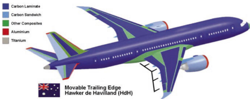
Fig. 5.2 Usage of composites in Boeing 787 Dreamliner structure [67]. Reprinted by permission from Elsevier
