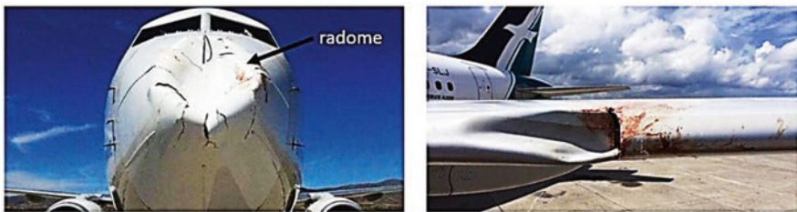
Fig. 2.25 Wildlife strike to an aircraft, damaging its radome and leading edges [119, 120]. Courtesy of The Aviation Herald
