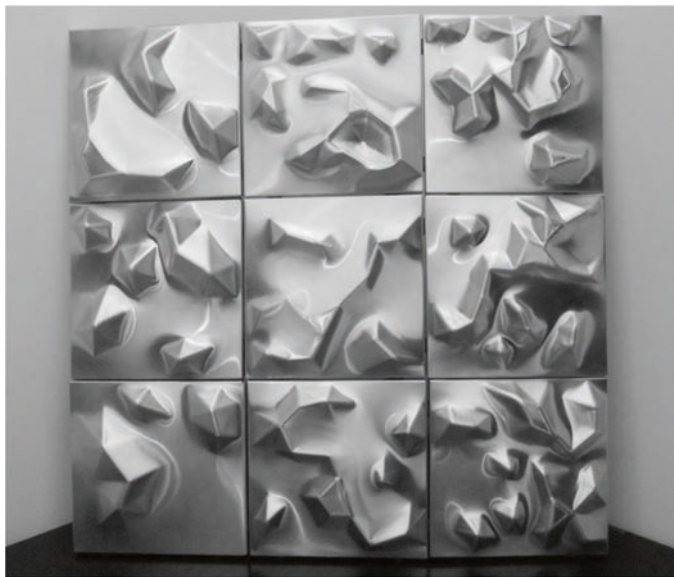
Fig. 12.8 SPIF manufactured decorative elements for facades
