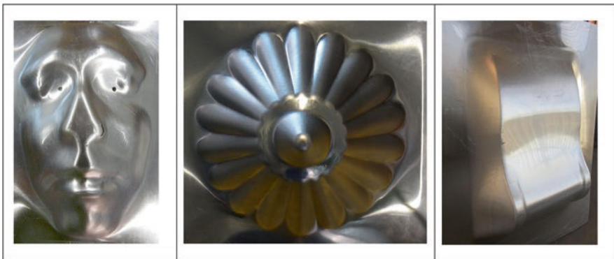
Fig. 12.5 Rapid prototyping and customized products from ISF
