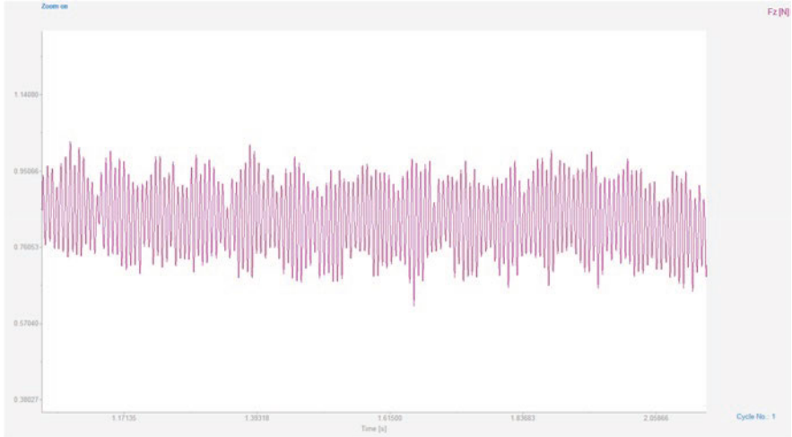
Fig. 11.12 Z-direction cutting forces in traditional milling (finish cut)
