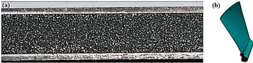
Fig. 2.28 (a) A metal foam sandwich panel (17-4 PH stainless steel foam core + 17-4 PH face sheets). (b) The engine fan model where the sandwich panel was used and numerically analyzed [123]. Reprinted by permission from SAGE
