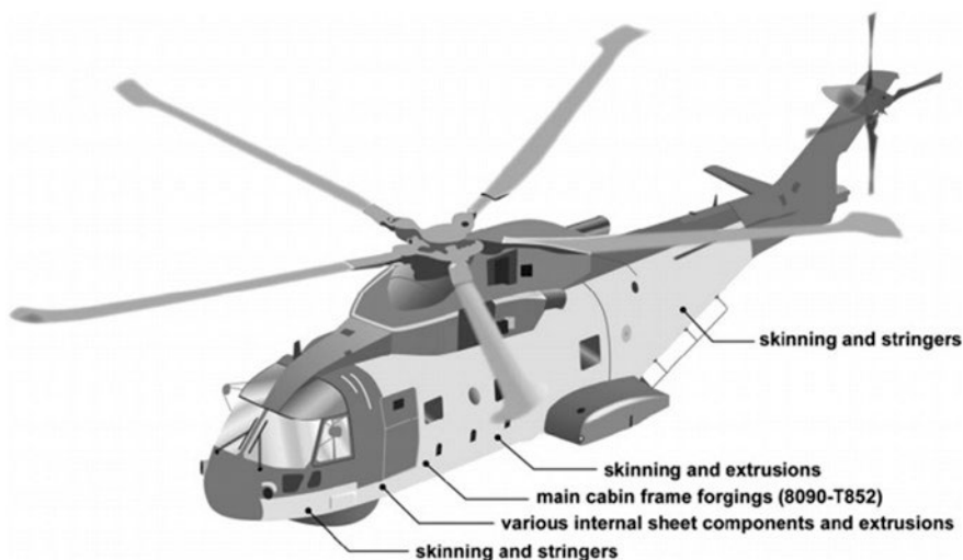
Fig. 1.3 8090T852 alloys as structural parts on the Agusta Westland EH101 [14]. Reprinted by permission from Elsevier
