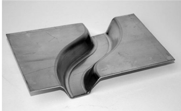
Fig. 12.12 Tunnel-type parts using ISF technology
