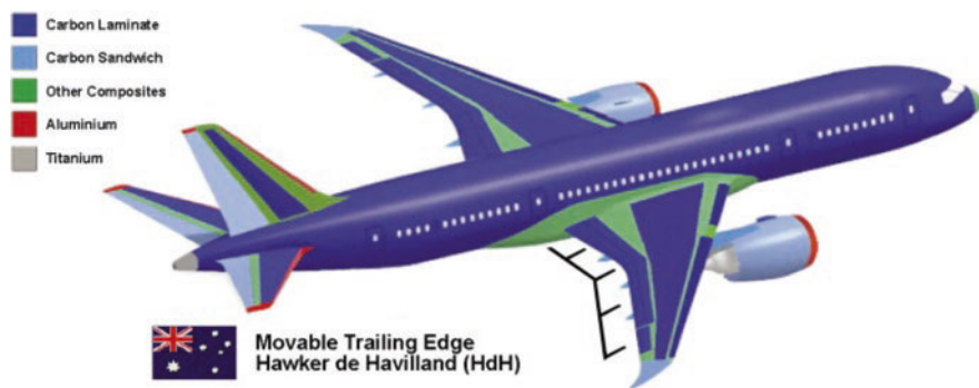
Fig. 5.2 Usage of composites in Boeing 787 Dreamliner structure [67]. Reprinted by permission from Elsevier
