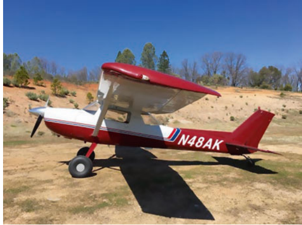
Fig. 7.7 Spring steel strut [5]. Reprinted by permission from Skywagons website
