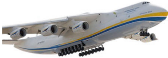
Fig. 7.4 Antonov AN-225 aircraft using tandem type landing gear to reduce the loads on the wheels
