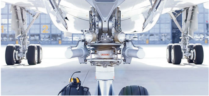
Fig. 7.1 The landing gear of the aircraft standing in the parked position on the ground [1]. Reprinted by permission from Lufthansa Technik AG
